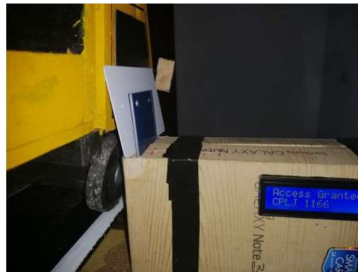
Figure 14 IOT device model- the process of reading the RFID: UID to grant the sand truck and displaying the 16*2 LCD display.
