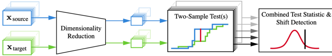
Fig. 4. Illustration of the process to detect data set change. Source and destination data are fed through a dimensionality reduction process and subsequently analyzed through statistical hypothesis testing [16]
