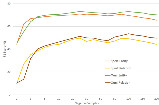
Fig. 3. The Variation of F1 Scores for Entity and Relation Classification between Our Model and SpERT Model under Different Negative Sample Quantities.
