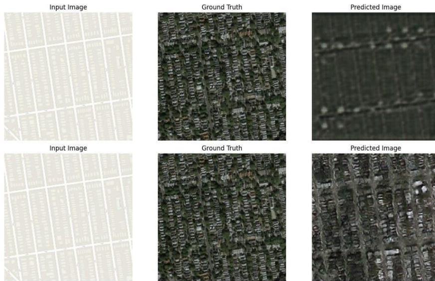
Figure 6. Output generated by Pix2Pix GAN after training for 1 epoch (top) and 100 epochs (bottom) on maps dataset.
