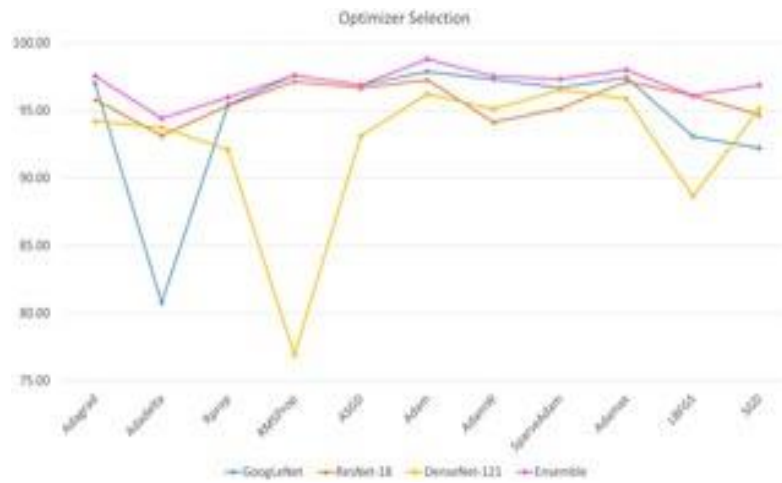
Fig 11. Variation of accuracy rates on the Kermamy dataset [2]) was achieved by the three base learners, GoogLeNet, ResNet-18, and DenseNet-121, and their ensemble, according to the optimizers chosen for fine-tuning.
