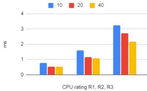
Fig. 6. Kyber-1024 multi-recipient key encapsulation performance in ms. on vCPU with R1=1000, R2=2000, R3=4000 single thread performance rating, for 10, 20, 40 public keys.
