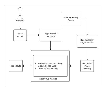
Figure 4. CI/CD pipeline structure
