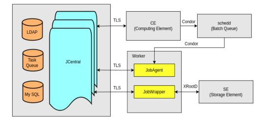
Figure 1. Architecture diagram of the emulated setup
