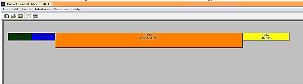
Figure (14): The four MODBUS frame fields in the OPNET program.
