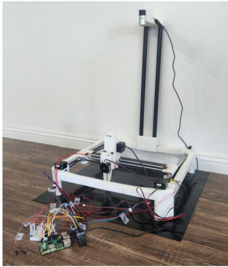
Figure 2. The completed system, including the Raspberry Pi 5, webcam, and H-bot gantry used for sorting
