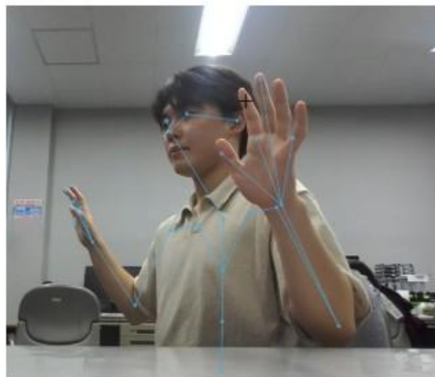
Fig.9: A captured frame showing a human posed detected in an image with the human skeleton keypoints
