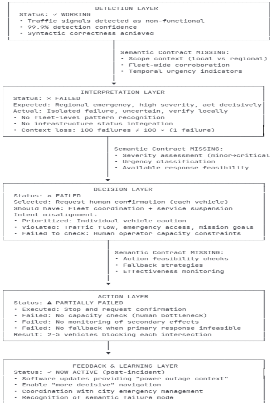
Figure 3: Semantic failure propagation through Waymo's autonomous vehicle architecture during the San Francisco power outage.
