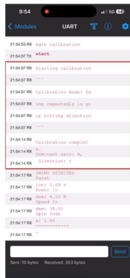
Figure 2. UART Communication Interface Used For Device–Application Data Transmission
