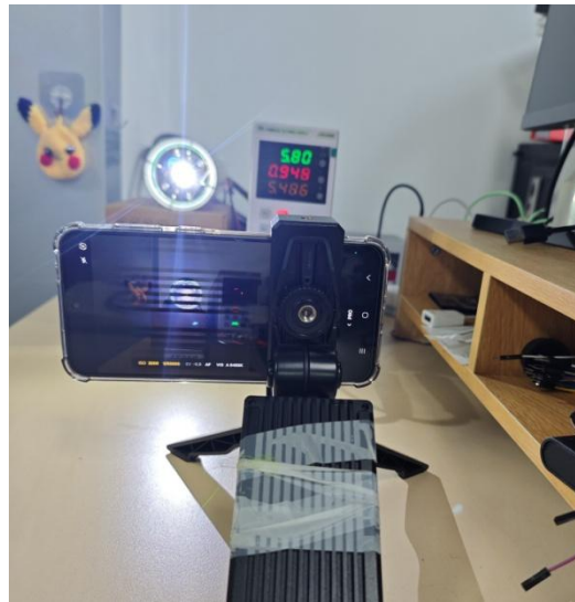
Fig.2. Testbed demonstration of the blooming effect in smartphone-based OCC.
