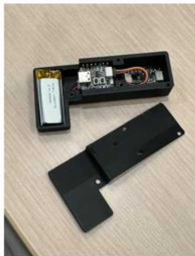
Figure 2. Hardware Architecture of the Dual IMU Sensor Pods
