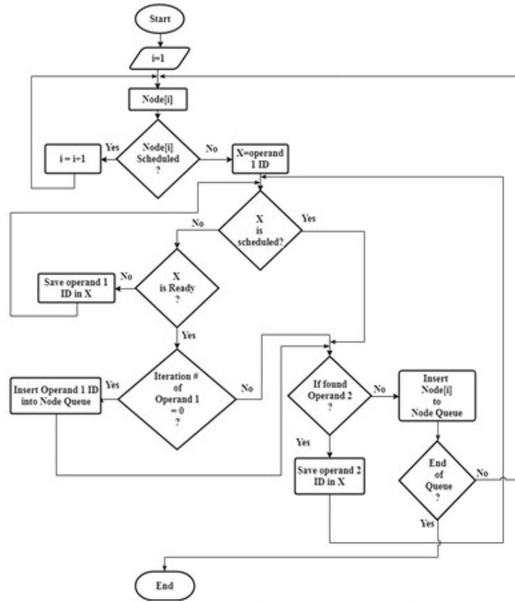
Figure 1: Flowchart of node queue construction
