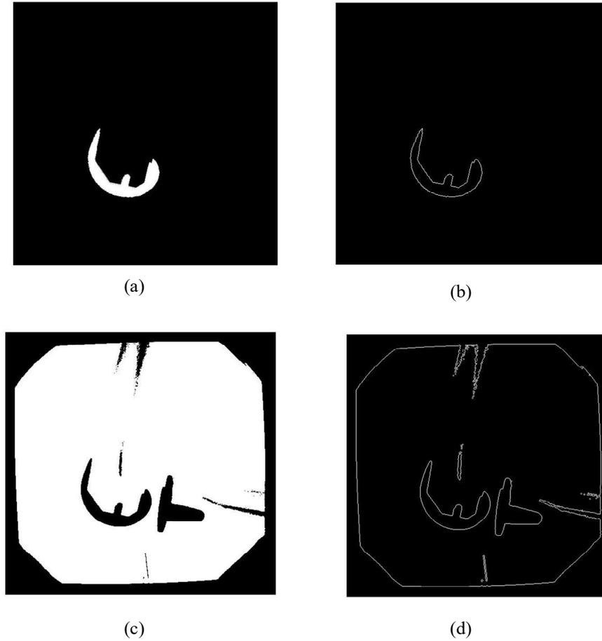
Figure 4. (a) and (c) show a 2D projected image of a 3D model of a femoral knee component and its corresponding fluoroscopy image respectively after the binarization process. (b) and (c) show the images after removing interior pixels of the femoral and tibial components.
