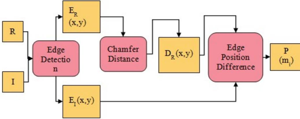
Figure 2. A simplified flowchart for calculating the EPD similarity measure.
