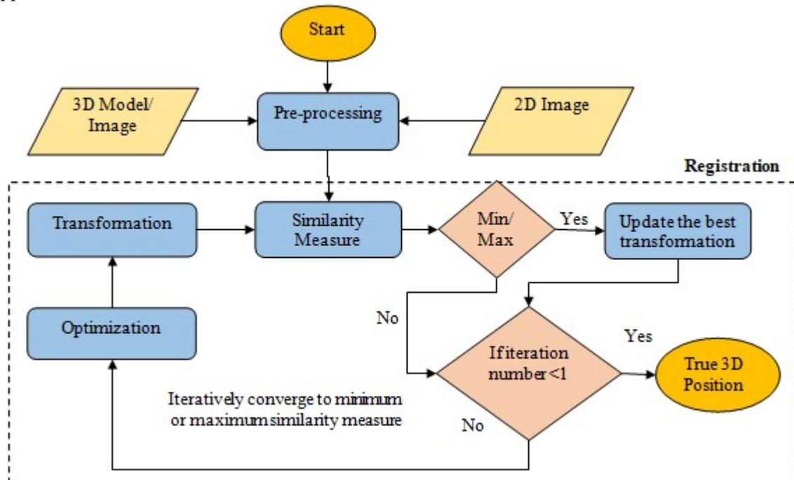
Figure 1. A simplified flowchart as an example for a 3D to 2D image registration.
