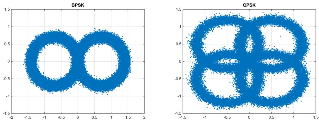
Figure 3: Output constellations for the sum of two BPSK signals and the sum of two QPSK signals with equal amplitudes
