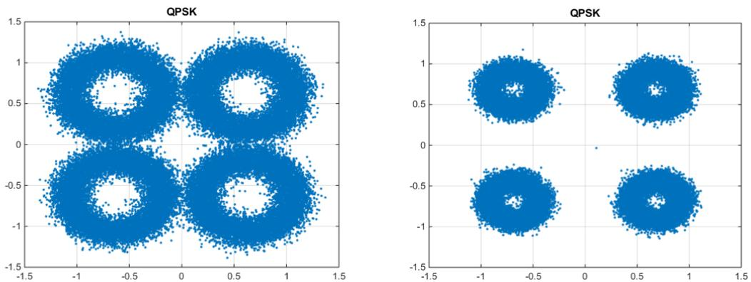
Figure 4: Output constellations for the sum of two QPSK signals with a ratio of amplitudes 2 and 4 respectively
