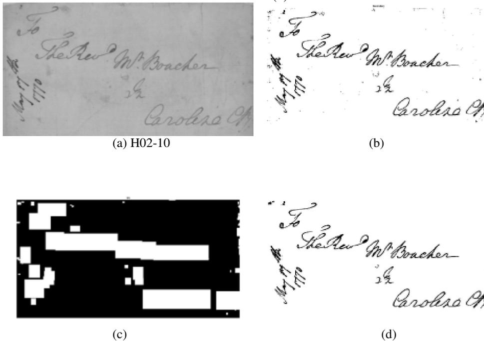
Figure 8. Noise removing for a low contrast image: (a) The gray scale image. (b) The binary image. (c) The rectangles fit each object in BI. (d) FI.
