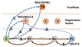
Figure 5. Register and Authentication Procedure
