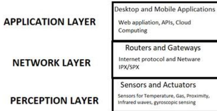
Figure 1. Basic Architecture of IoT devices
