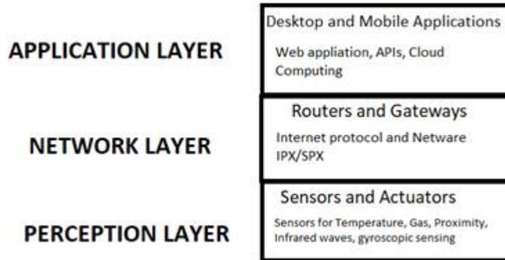
Figure 1. Basic Architecture of IoT devices
