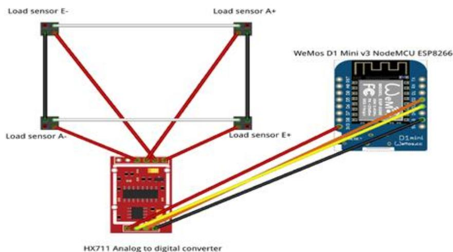
Figure 7. Wiring and Setup of the Components
