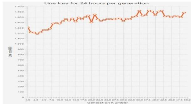
Figure 8: Total line loss for 24 hours with power scheduling and network reconfiguration
