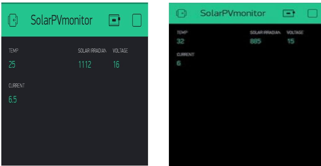
Figure.10 Real-time Solar PV monitoring system using Blynk
