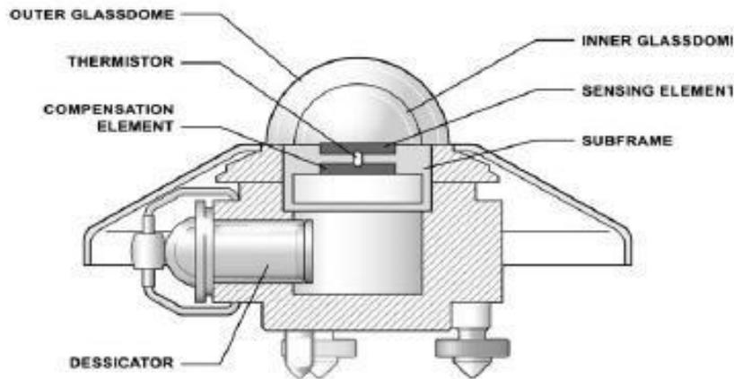
Figure 6. The general structure of CM21 Pyranometer
