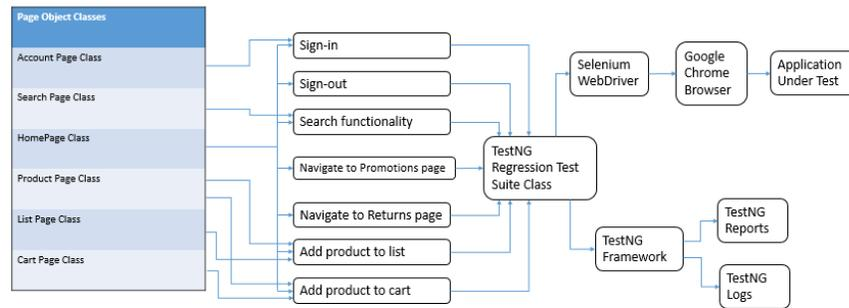
Figure 1. Proposed Regression Test Suite Automation Framework
