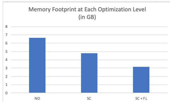
Figure 7. Memory Footprint at Each Optimization Level
