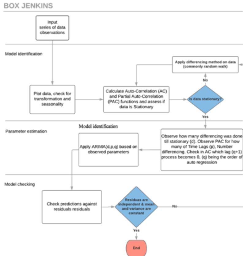
Figure 1. Box Jenkins iterative fitting model
