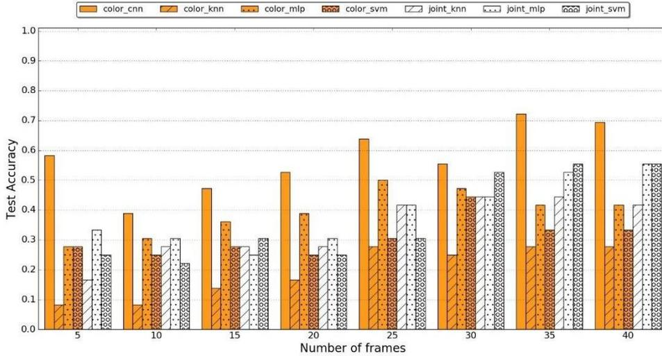
Figure 6 Performance of all types of predictors using different input data format, trained and tested on different datasets. Orange bars indicate predictors trained with color image data, white bars indicate predictors trained with joint data.
