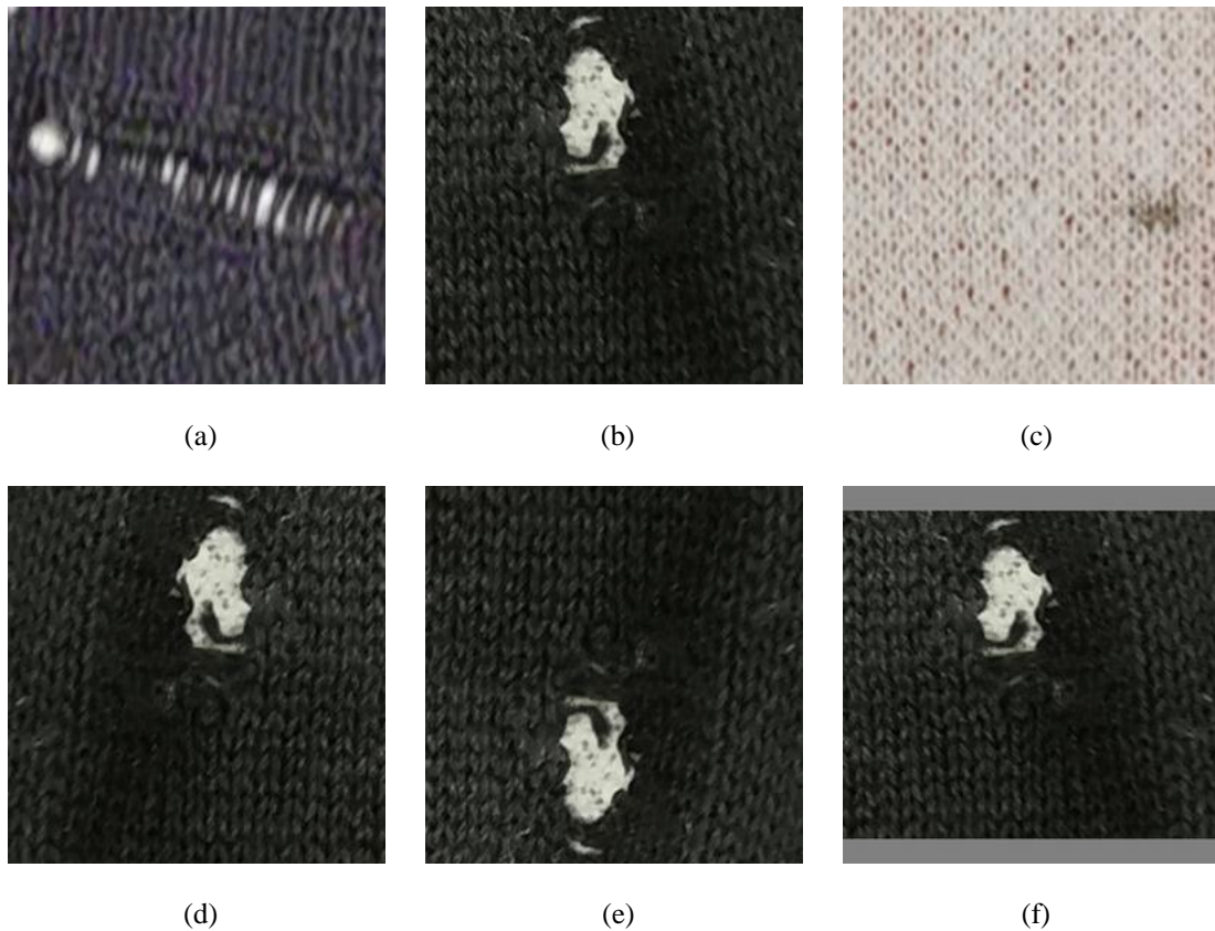
Fig 1. The examples of fabric defects image and augmentation results. (a) is drop needle. (b) is broken hole. (c) is fly yarn. (d) and (e) are (b) flipped in horizontal and vertical direction, (f) is (b) distorted and resized in standard size.
