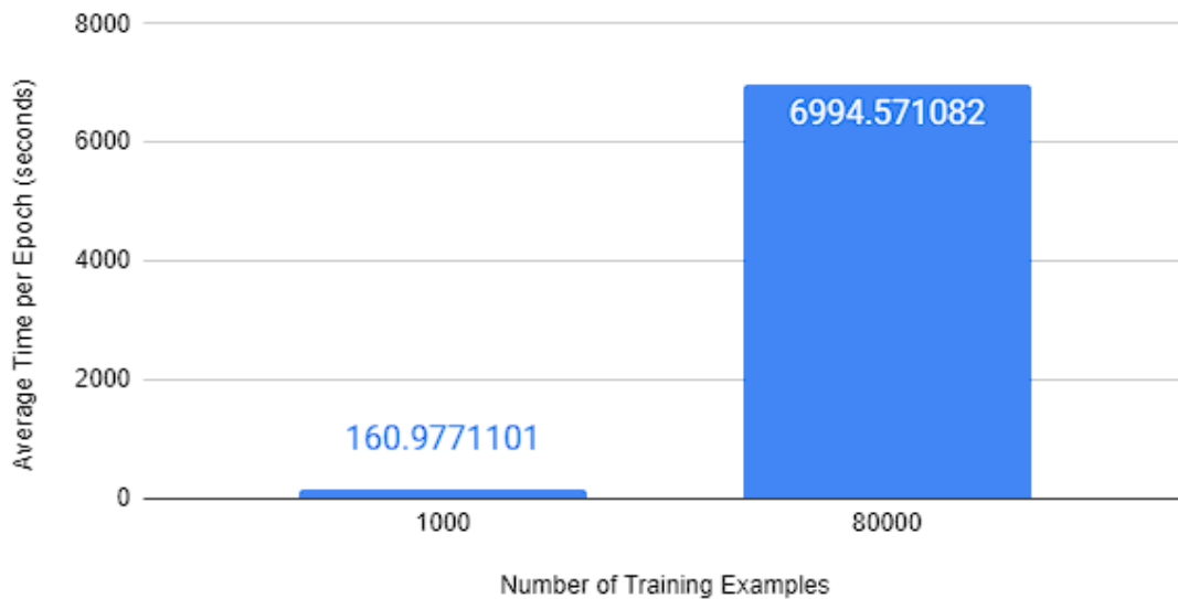
Figure 8. Comparison of the average time per training epoch (in seconds), for experiments run with 1,000 and 80,000 training examples.
