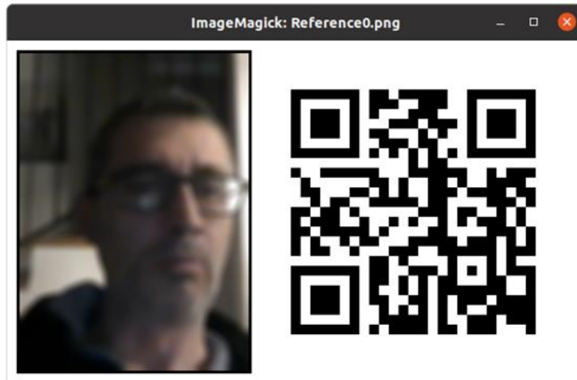
Figure 2: photoQR ID card produced by the creation step of the algorithm with image blurring option enabled. The right part of the card contains the QR with data produced by the image hashing function of the left picture.
