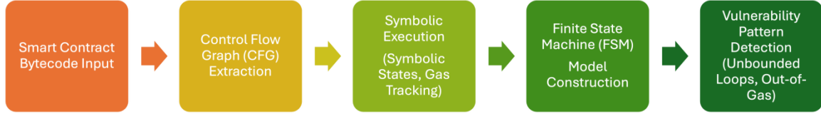
Figure 2. Technical Workflow Diagram of MadMax Static Analyzer
