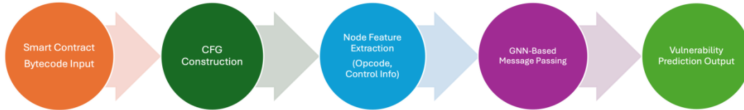
Figure 4. ContractGraph Workflow for Vulnerability Detection
