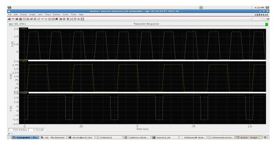
Fig 16(a): OR gate I/O waveforms
