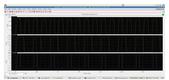
Fig 16(b): AND gate I/O waveforms
