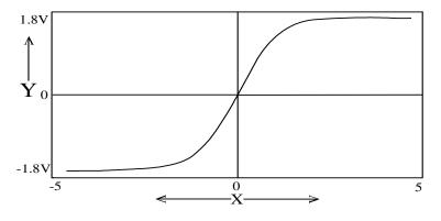
Fig.6 DC response of CMOS Differential Amplifier
