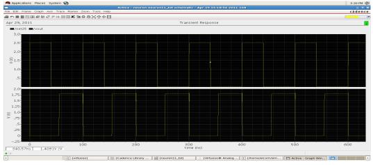
Fig 16(c): NOT gate I/O waveforms
