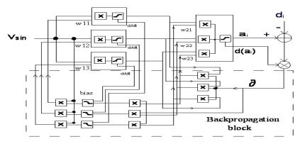
Fig.7 Neural network (1:3:1) with Backpropagation Algorithm
