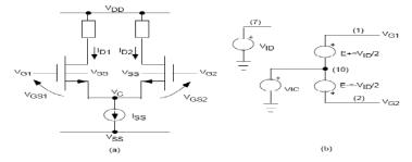
Fig.4 General MOS Differential Amplifier: (a) Schematic Diagram, (b) Input Gate voltage implementation.
