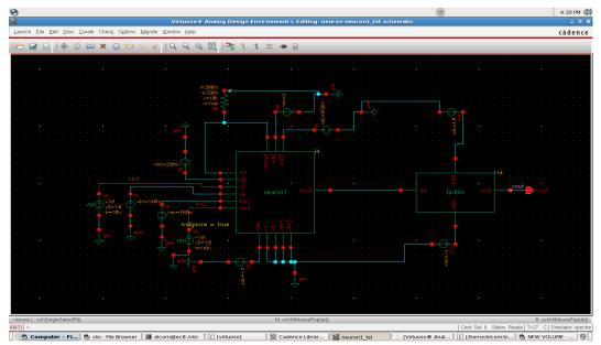
Fig.15 Test bench for digital operation
