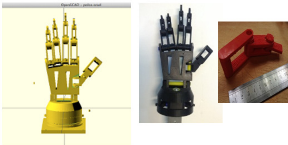
Figure 1: Modelling process: OpenSCAD design and 3D printout. Example of modular finger is on the right.
