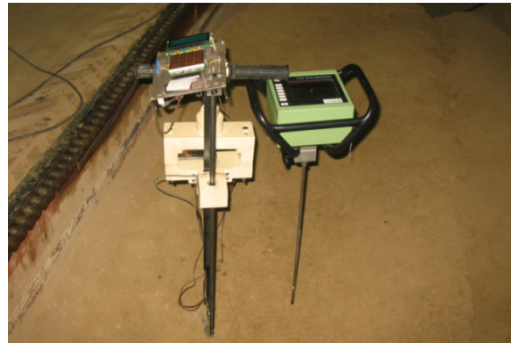
Figure 4 built device in left and commercial type in right both in soil tank
