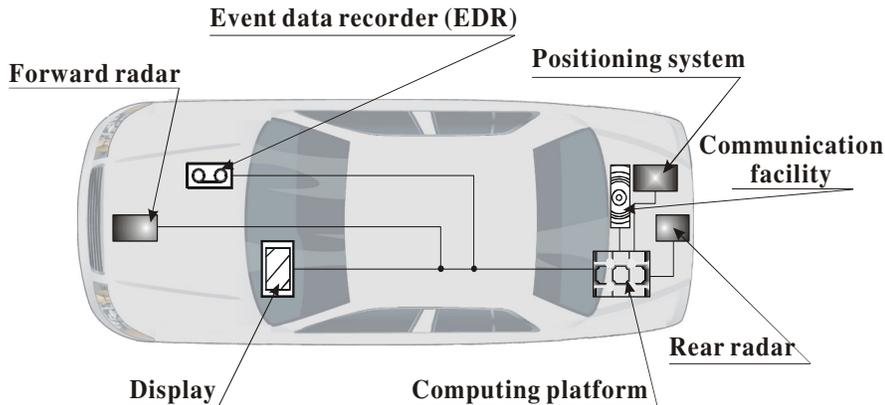
Fig. 1. The structural components of VANET node
