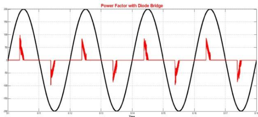
Fig.11. Simulation output wave form of Power factor with Diode Bridge Rectifier based SRM
