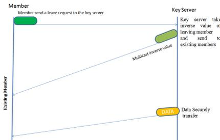
Figure 3: Leaving Process of Proposed Approach
