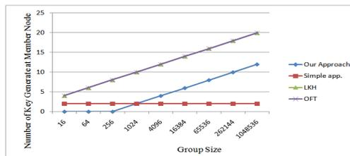
Figure 5(b): Key Generation Overhead at the Member Node during Leave Process
