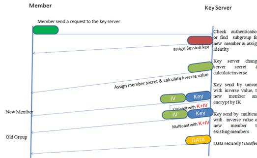
Figure 2: Joining Process of Proposed Approach
