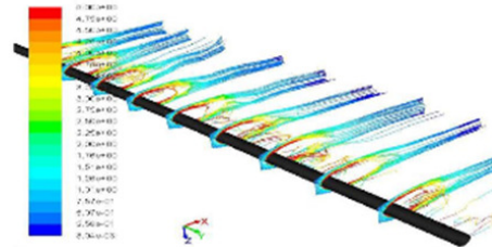
Fig.10 Path lines colored by vorticity magnitude (IFS model)
