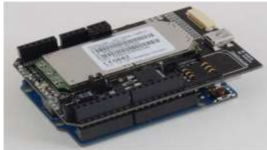
Fig. 2. Arduino interfaced with 3G shield.
