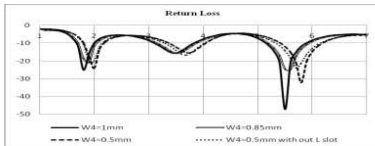
Figure 8: S11 versus Frequency observations for different gaps ( W_4 )
