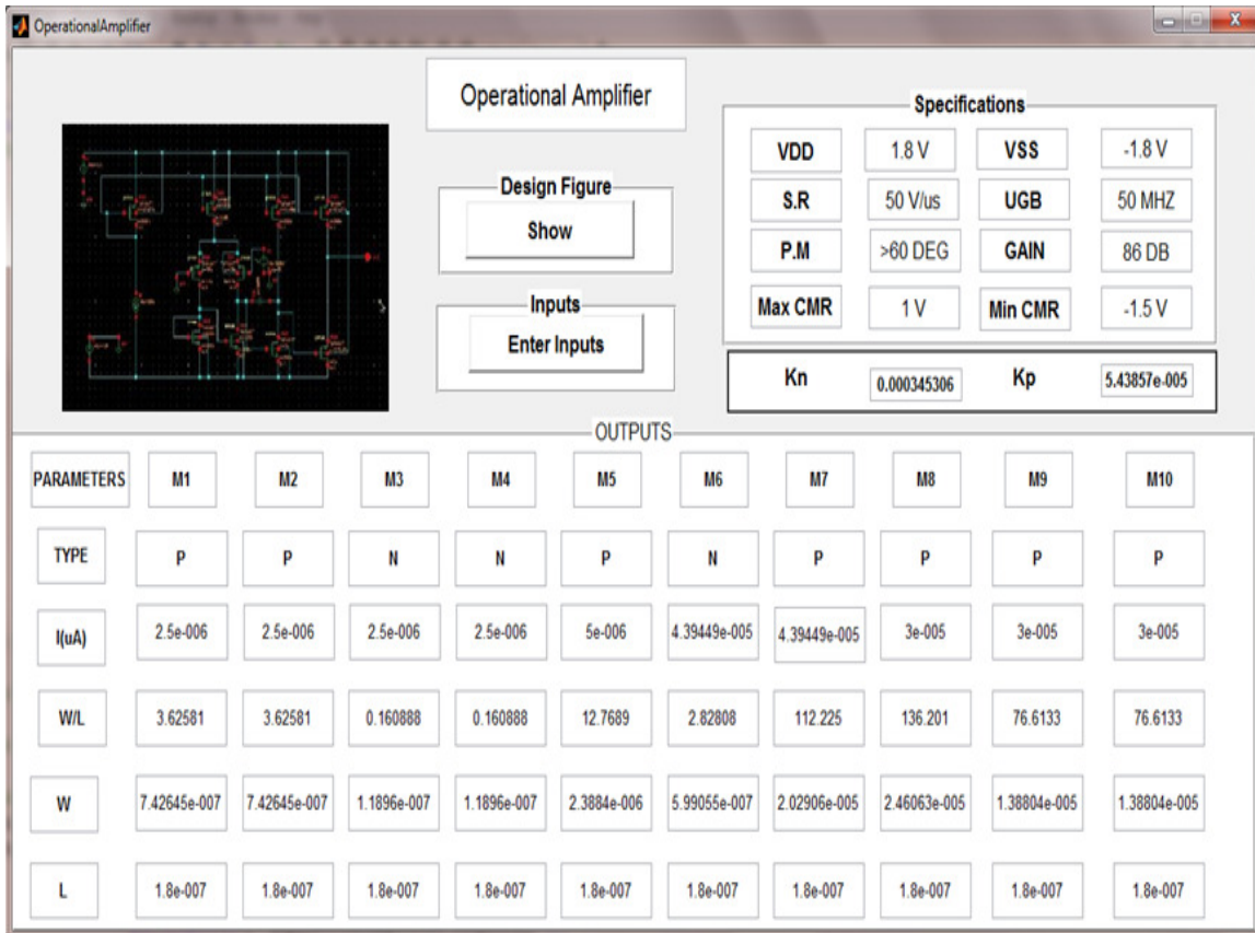
Fig.5 output window with W/L values of the 2 stage op-amp
