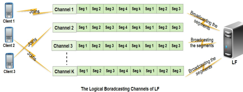
Figure 2. Logical broadcasting channels of the LF
