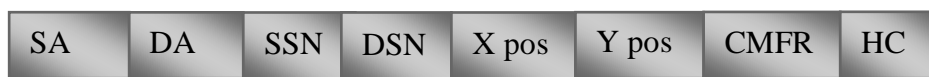
Figure 1: RREQ Packet Format (SA-Address of Source, DA - Destination Address, SSN : Source Sequence Number, DSN - Destination Sequence Number, X pos - position of X, Y pos -position of Y , CMFR- Cost Metric of Forward Route, HC - Hop Count)
