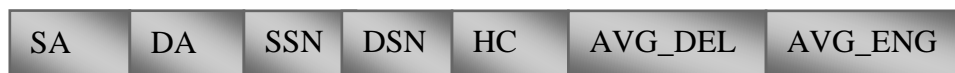
Figure 3: RREP Packet Format (SA- Address of source, DA - Destination Address, SSN : Source Sequence Number, DSN - Destination Sequence Number, , HC - Hop Count, AVG_DEL - Average Delay, AVG_ENG- Average Residual Energy)
