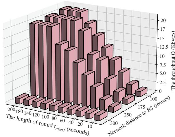
Figure 2. The throughput  $Q$  with modification  $t_{round}$  and network distance to the base station
