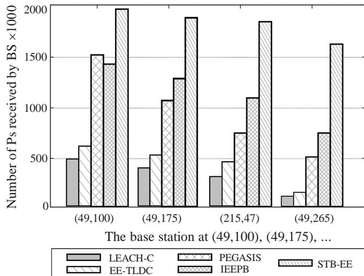
Figure 8. The amount of data packets received successfully by BS when positioning modifies
