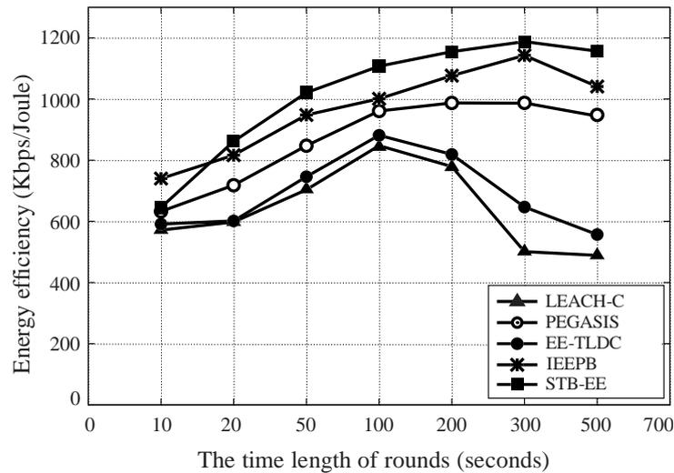
Figure 9. The energy efficiency per throughput with changing the time duration of rounds
