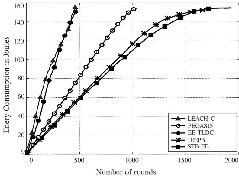
Figure 6. Total energy consumption of the network per round with BS position at (50,175)
