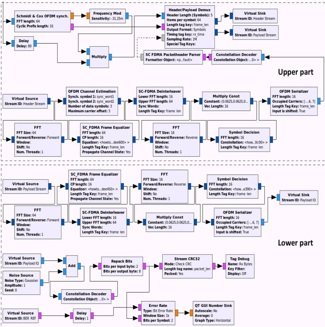
Figure 6. Flow graph of DSA UL-LTE configuration with SC-FDMA demodulator
