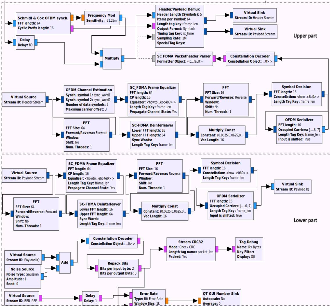
Figure 4. The demodulation of UL-LTE setup SC-FDMA
