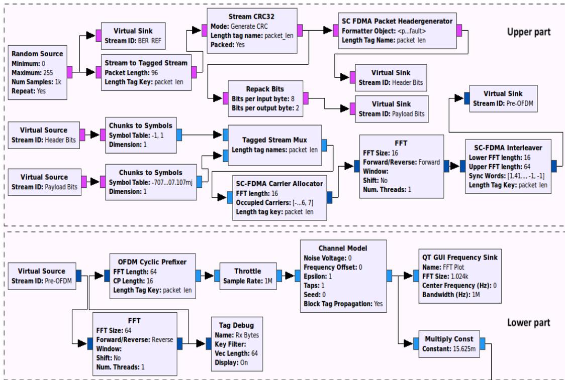
Figure 3. The modulation of UL-LTE setup with SC-FDMA
