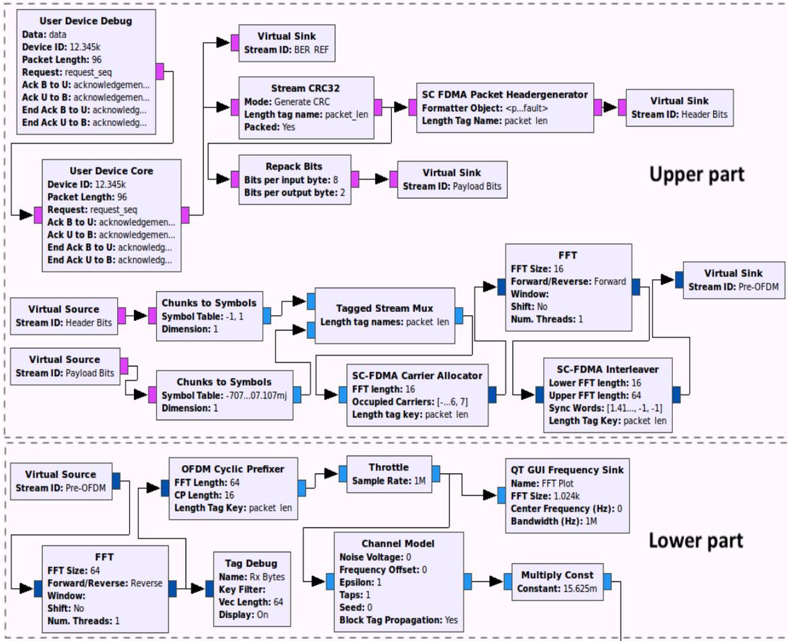
Figure 5. Flow graph of DSA UL-LTE configuration with SC-FDMA modulator
