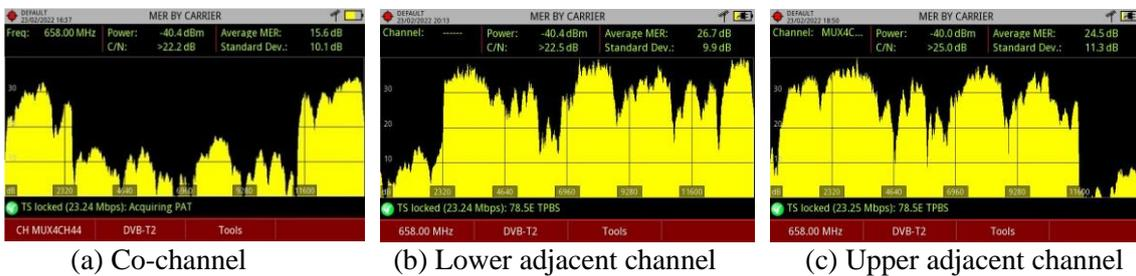
Figure 19. MER (Modulation Error Ratio) by Carrier Measurement
