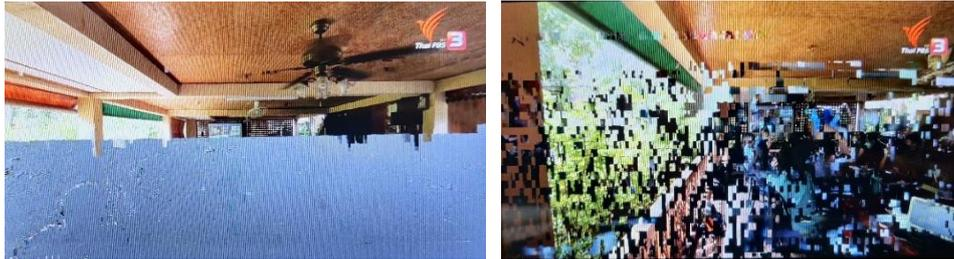
Figure 16. Examples of Video Distortion on TV screen (black and keep freezing)
