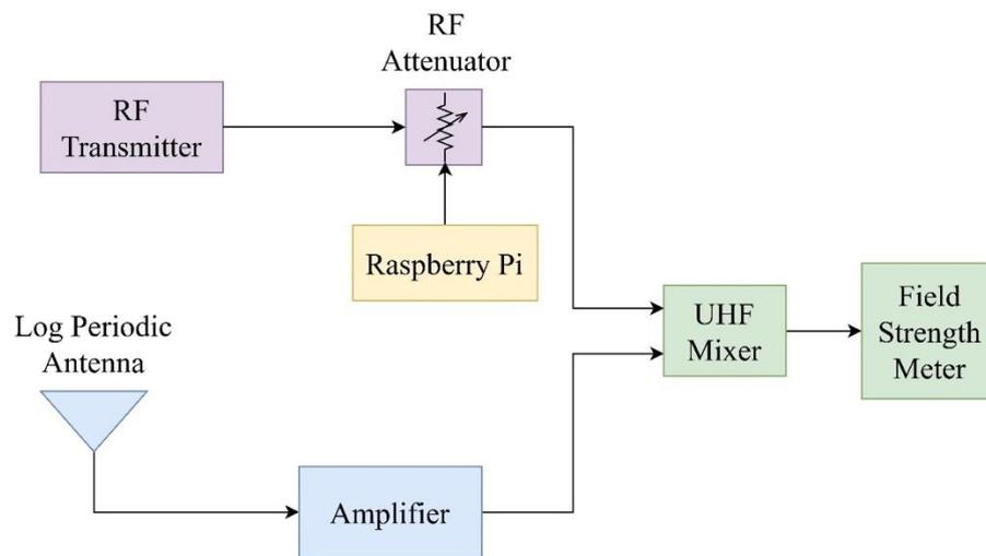
Figure 6. Block Diagram of the Testbed
