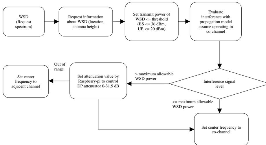
Figure 5. Block Diagram of the Proposed Algorithm implemented in our Hardware
