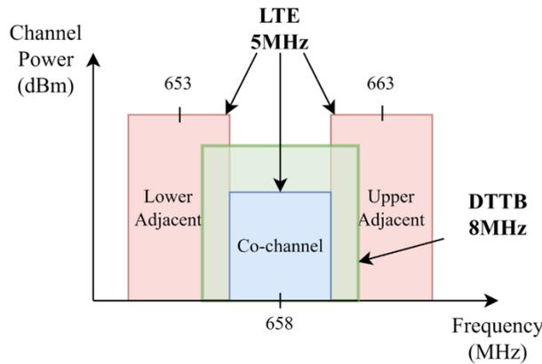
Figure 3. The Coexistence Scenario between DTTB and LTE Signal
