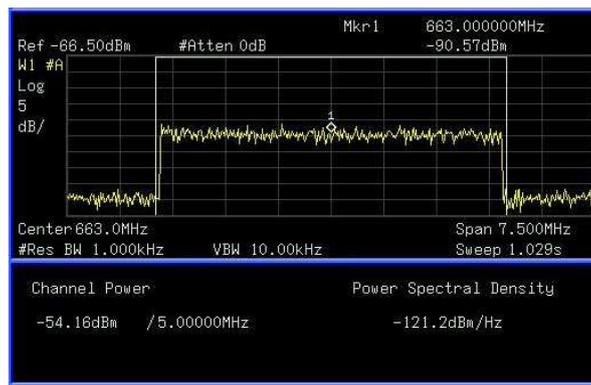
Figure 9. The LTE Signal with 5MHz Bandwidth measured by KEYSIGHT N9320B Spectrum Analyzer.
