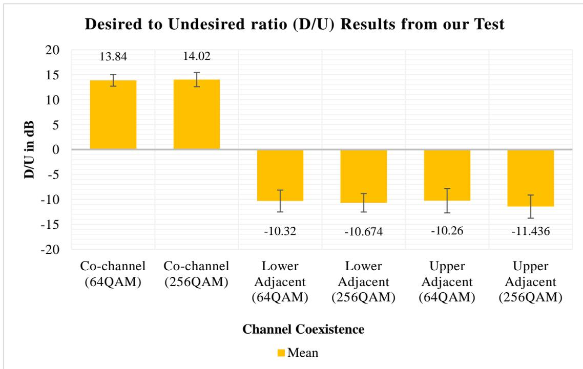
Figure 14. D/U Ratio Results from our Test
