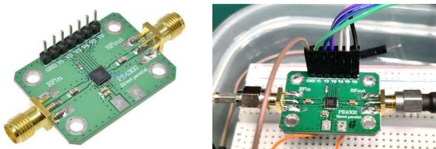
Figure 10. The RF Attenuator
