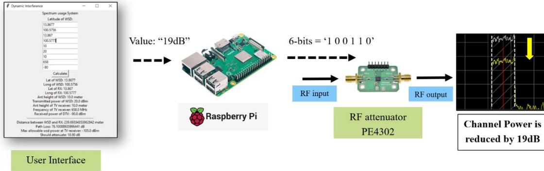
Figure 13. Algorithm Processing with Testbed Hardware.
