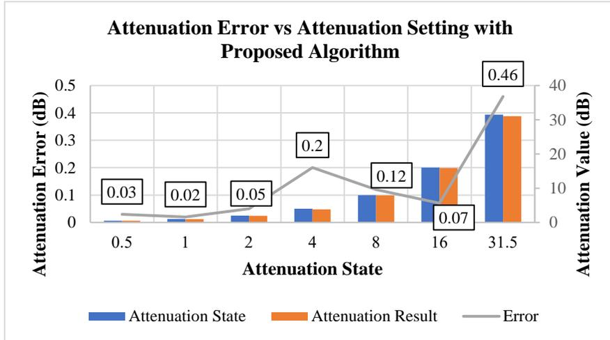
Figure 18. The graph of Attenuation Error vs Attenuation Setting
