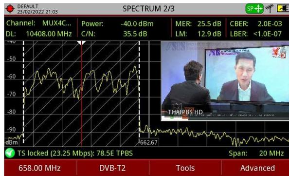
Figure 8. The received DTTB Signal of 8MHz Bandwidth at Frequency of 658MHz measured by a PROMAX Field Strength Meter.
