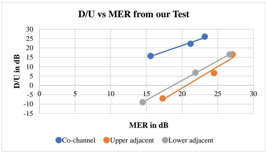
Figure 20. The Graph of D/U Ratio versus MER (Modulation Error Ratio)
