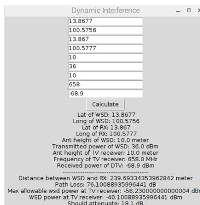
Figure 12. The GUI of the Dynamic Interference Suppression System
