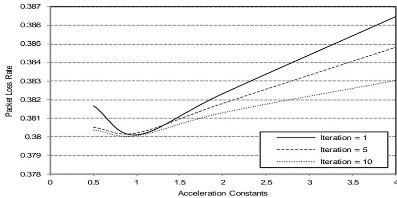
Figure 7. Packet loss rate for various acceleration constants in nine particles swarm
