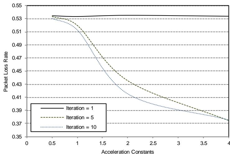
Figure 6. Packet loss rate for different acceleration constants in one particle swarm
