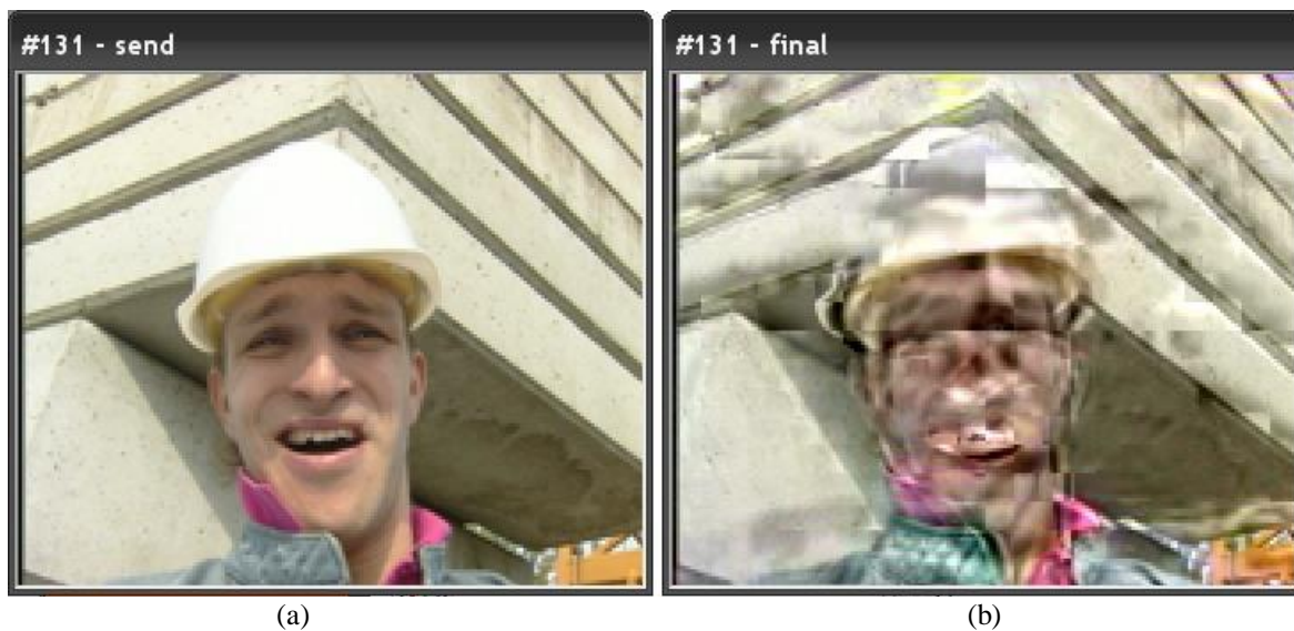
Figure 12. Displays the effect of the dropped packets on the receiver node. (a) the video at node 0 (sender); (b) the received video at node 3 (receiver).
