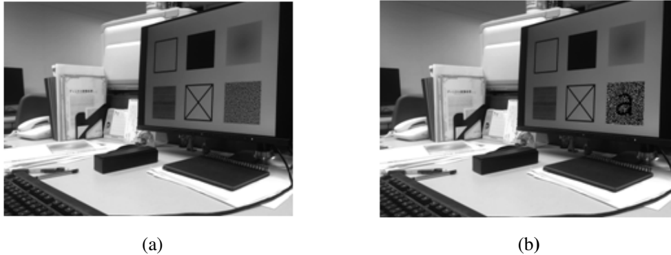
Figure 12. Example of actual image results using our method, showing (a) an input image with a hidden message and (b) the resulting image after automatic detection and decryption.
