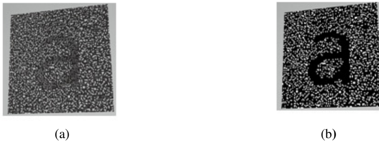
Figure 13. Illustrating our image correction method both (a) without applying the correction method and (b) with the correction method applied.
