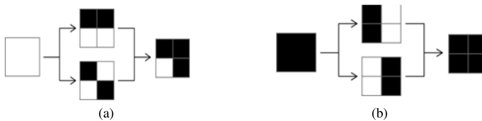
Figure 2. Encryption and decryption schemes for (a) white pixels and (b) black pixels.
