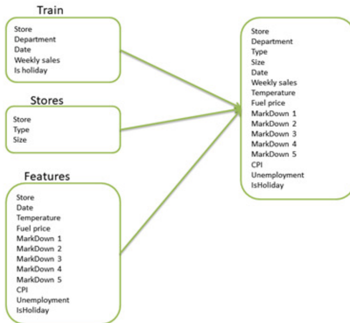
Figure 3. Fields of the original datasets and of the final one generated by the two “Join” operators.
