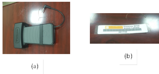
Figure 2. (a–b): The system components (RFID reader and tag)
