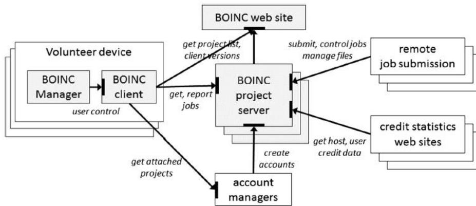
Figure 3. The components and RPC interfaces of the BOINC system [4]
