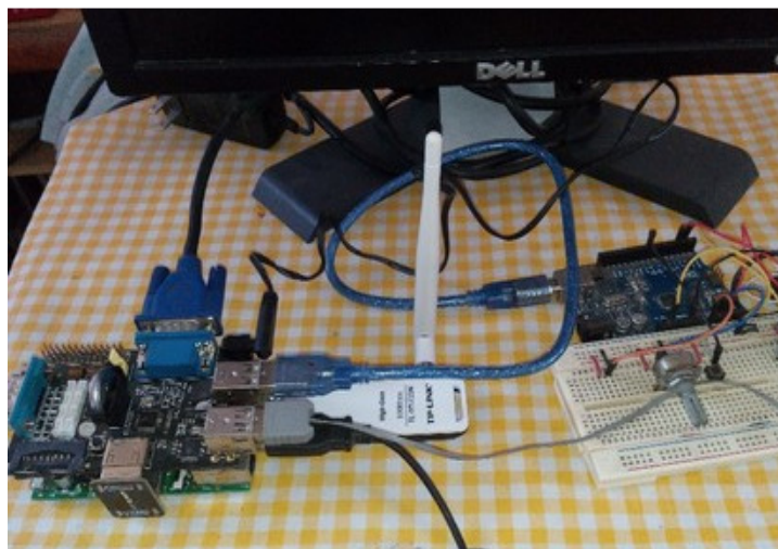
Figure 5. Raspberry Pi and Arduino UNO architecture
